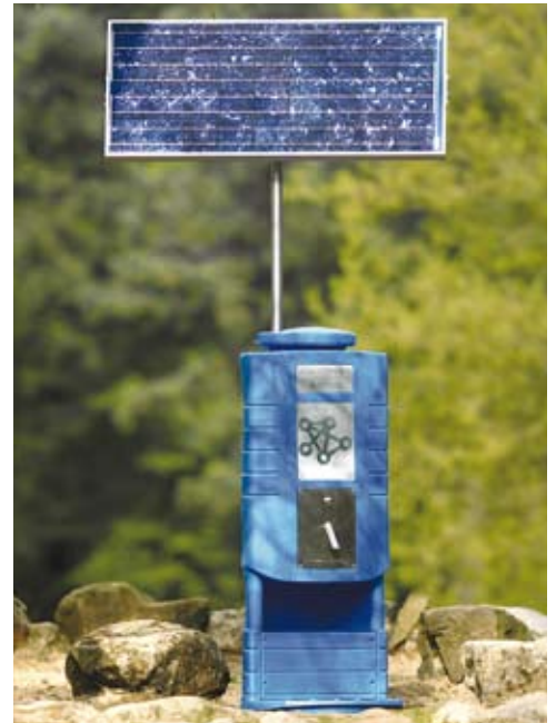
The Naïade solar-powered water purifier that Electron Solar has just begun distributing as part of its solar-power range. The system uses mechanical cloth filters and a UV reactor to produce safe drinking water for rural populations.
